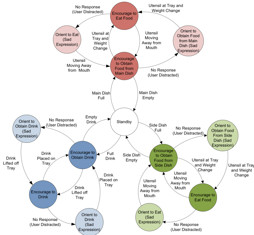
Figure 6. FSA diagram for the robot's assistive behaviors during the meal-eating activity.
